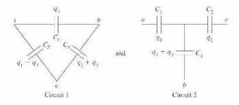
From Circuit 1:  $V_{ac} = \frac{q_1 - q_3}{C_y}$  and  $V_{bc} = \frac{q_2 + q_3}{C_x}$ , where  $q_3$  is derived from  $V_{ab}$ :
